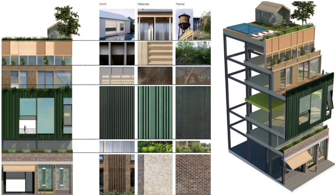
Figure 27 (above left): Truncated elevation. Figure 28 (above centre): The materials palette. Figure 29 (above right): Axonometric section, showing how the tiered façade steps in and out.
